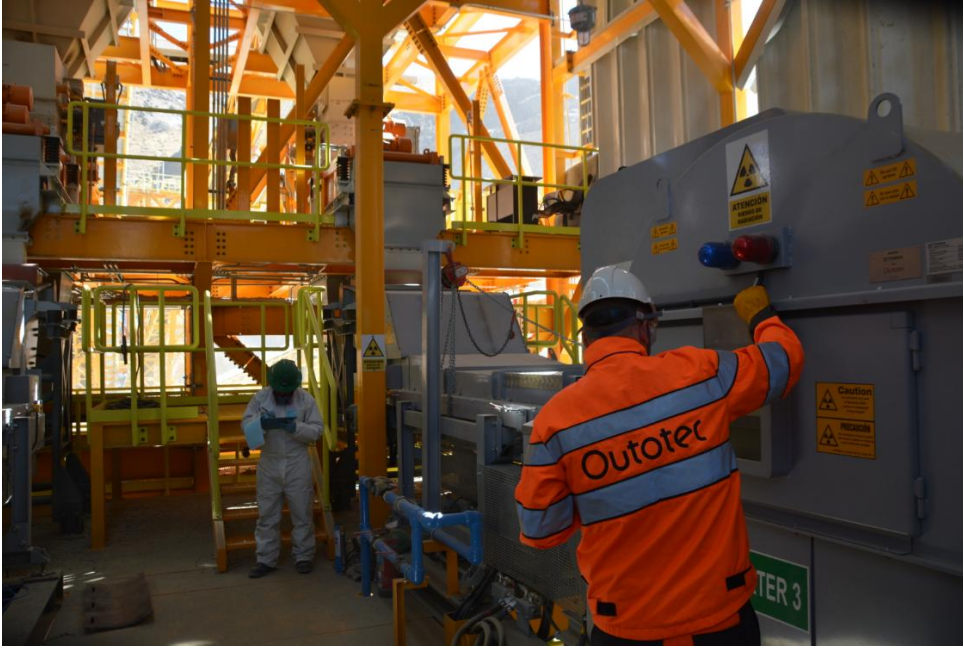
Figure 2 Commercial TOMRA COM Tertiary XRT ore sorting machine
