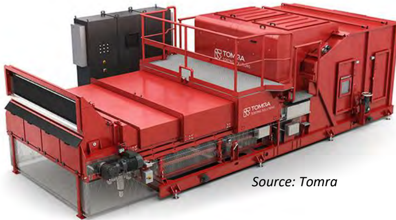
Figure 13-12: Tomra high capacity commercial XRT Ore Sorting Machine
