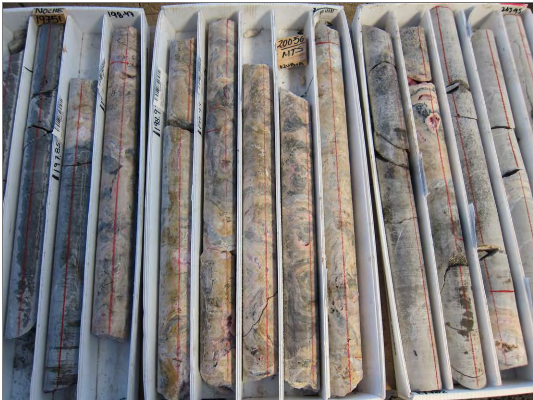
Figure 7-8 Example of Banded Veining of the Main Ixtaca Vein Swarm Zone of
