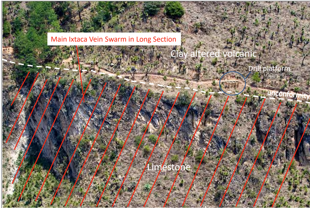
Figure 7-7 Photo of Cerro Caolin of the Main Ixtaca Vein Swarm From North Looking to the South Showing the Contact between the Clay Altered Volcanic and Limestone Units
