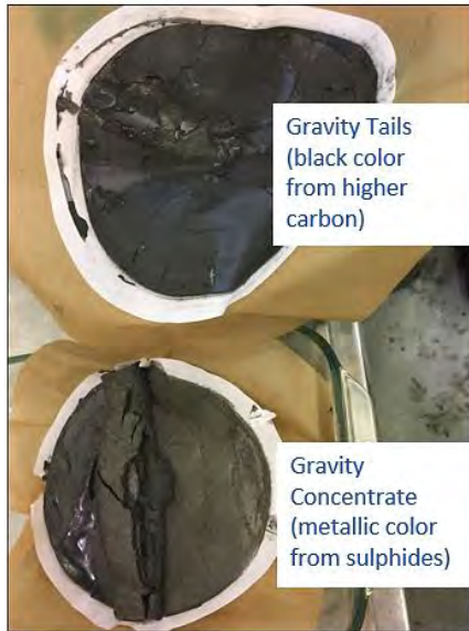
Figure 13-48: Black Shale – gravity concentration of flotation rougher concentrate
