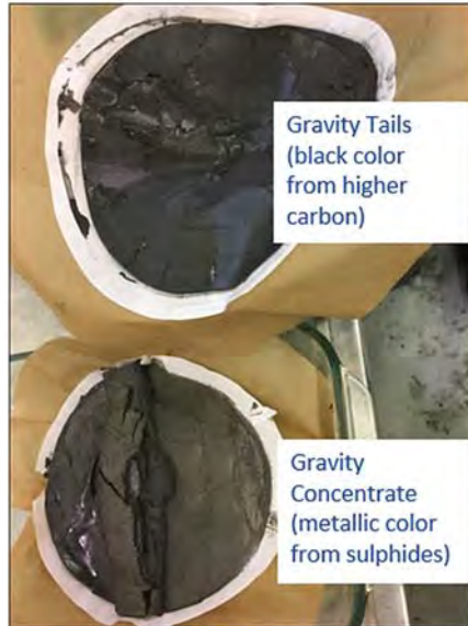
Figure 10-48: Black Shale – gravity concentration of flotation rougher concentrate
