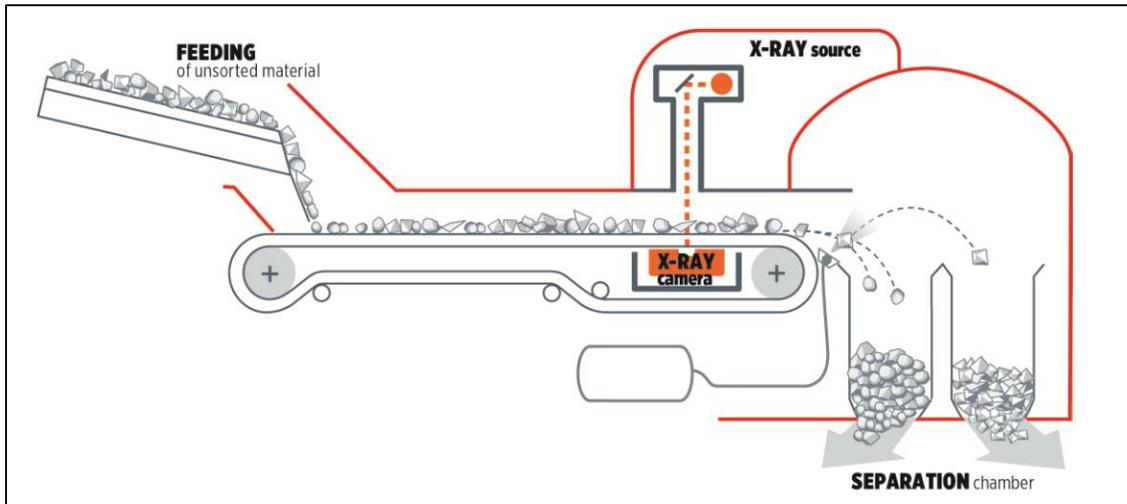
Figure 1 XRT Ore Sorting – functional principle
